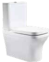
Cover close coupled fully enclosed WC & seat 6/3L* Cistern, dual flush fittings included 375(w) x 812(h) x 630(d)mm
